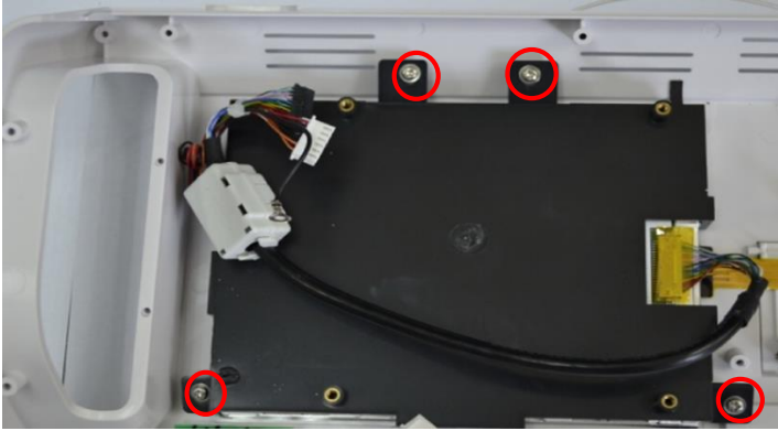
Fig. 9.3: Four screws securing the LCD display unit
