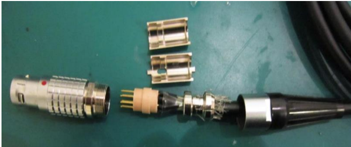
Fig. 4.3: Disassemble the plug and use 70% alcohol solution to wash each component
