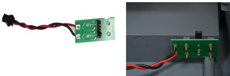
Fig. 4.1 Battery Interface Board Position Sketch Map
